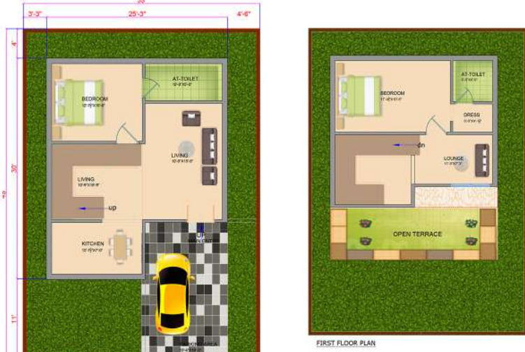
REVISED TYPICAL EAST FACING HOLIDAY HOMES CONCEPTUAL LAYOUT SLAB AREA G+1 :1400 SQ.FT PLOT AREA : 183 SQ.YRDS
