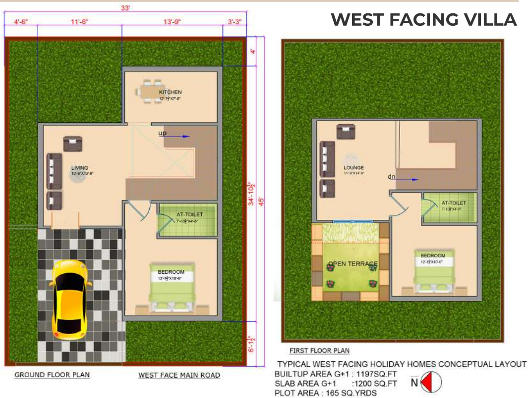
TYPICAL WEST FACING HOLIDAY HOMES CONCEPTUAL LAYOUT SLAB AREA G+1 :1197SQ.FT SLAB AREA G+1 :1202 SQ.FT PLOT AREA : 165 SQ.YRDS
