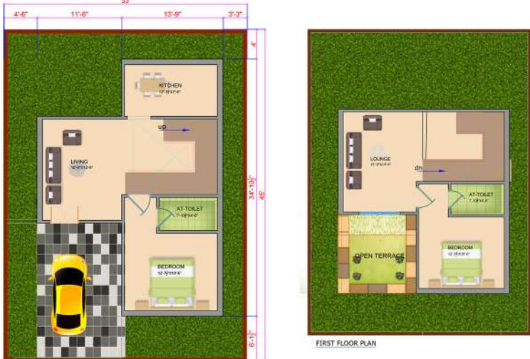
TYPICAL WEST FACING HOLIDAY HOMES CONCEPTUAL LAYOUT SLAB AREA G+1 :1400 SQ.FT PLOT AREA : 183 SQ.YRDS
